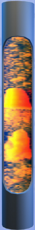
With Wire Mesh System visualized bubble flow.
